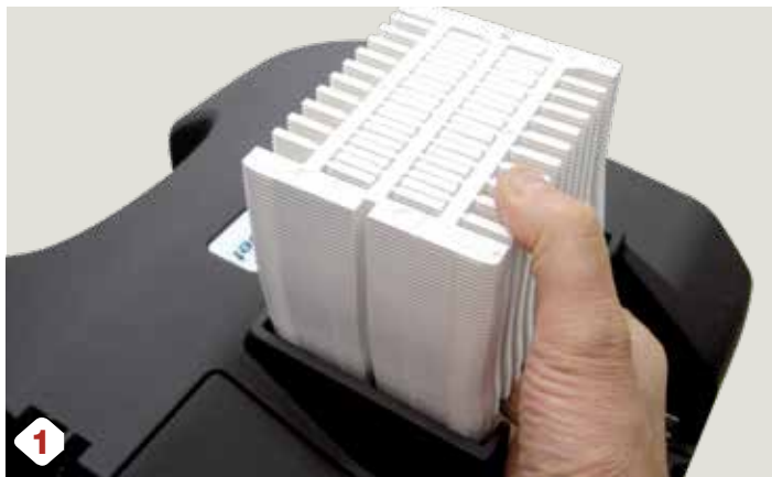
1 Insert the material in the feeder.
