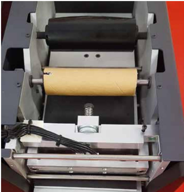
Inserting the ribbon
