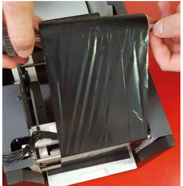
Winding and locking the ribbon
